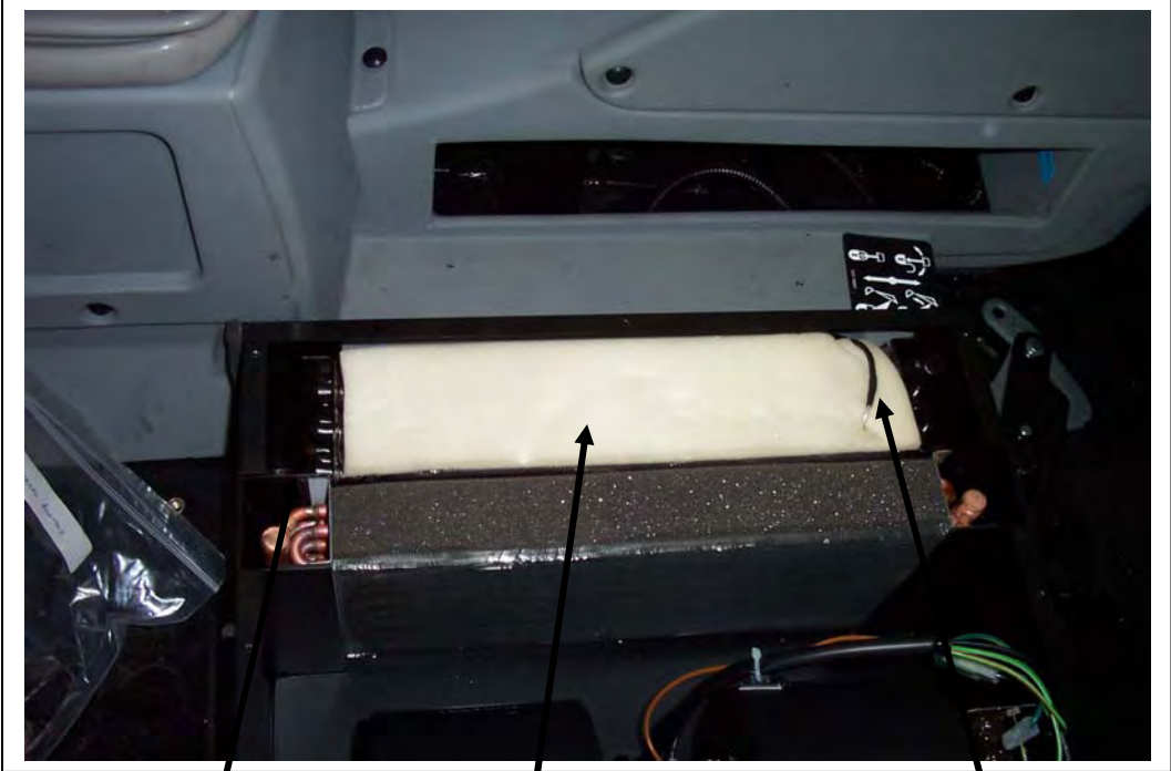
Thermostat probe installed between 1 st and 2 nd rows of tubes, 2" in from the fitting end of the coil about 6" deep
