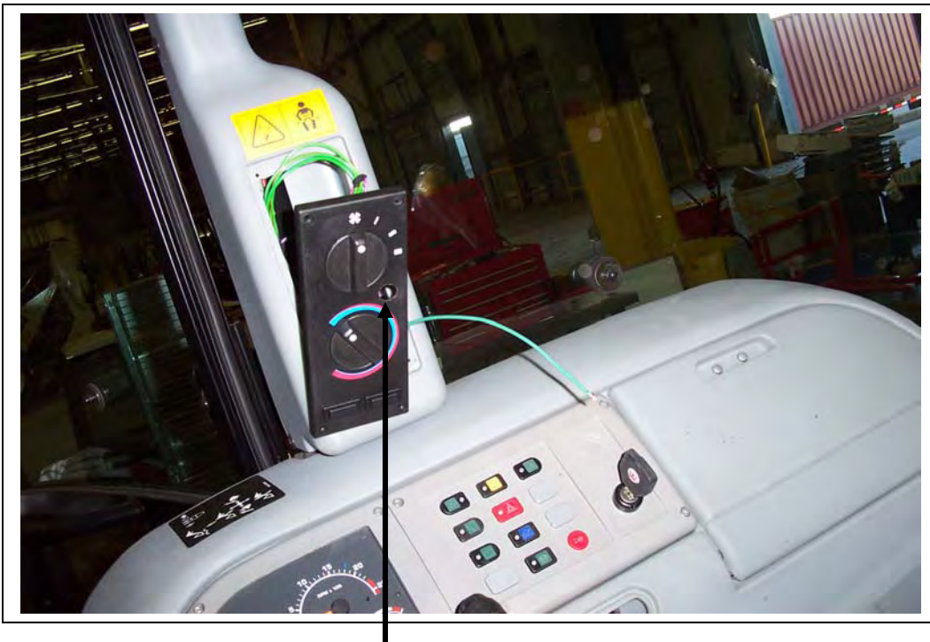
5/8" hole drilled for AC on/off pushbutton switch
