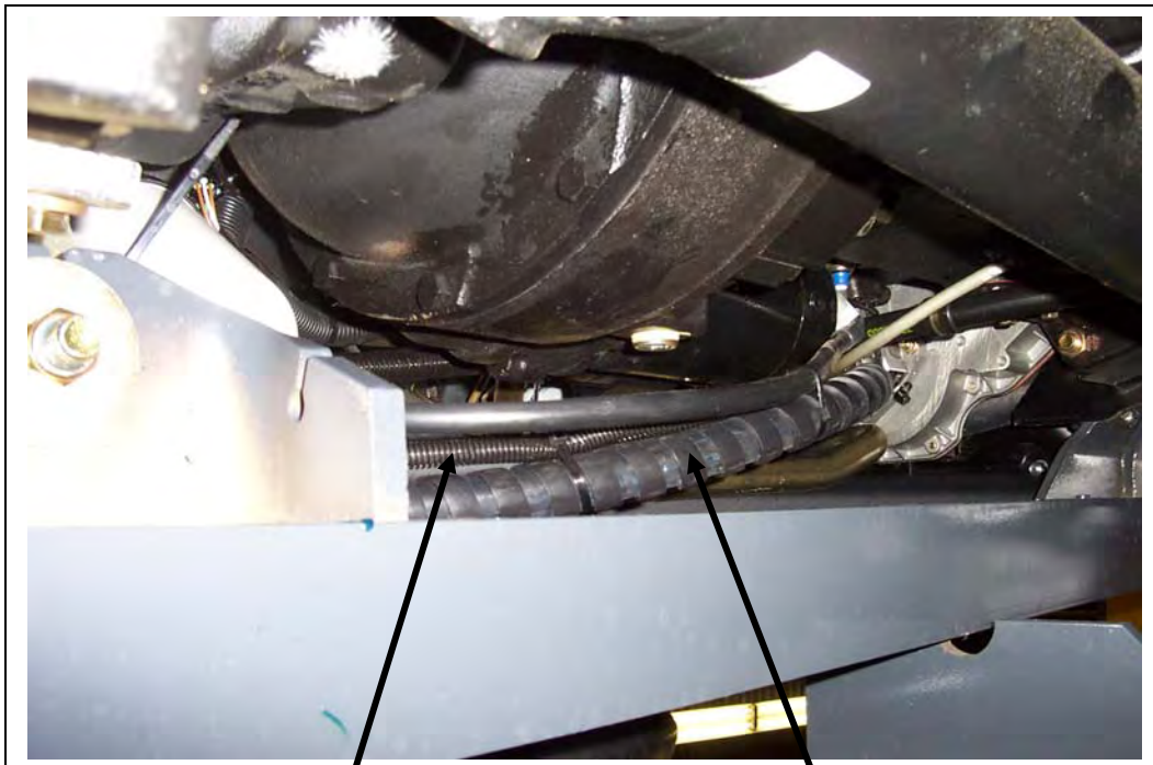
Clutch wire run along with 1/2" hose all the way to the heat/AC box
