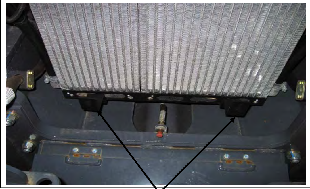
Lower condenser mount brackets installed loosely.
