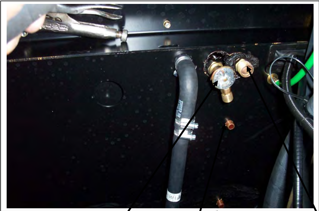
The expansion valve is turned about 90° to point forward and then tightened into place
