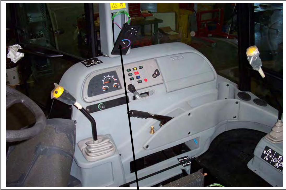
Heat/AC control panel unscrewed from frame
